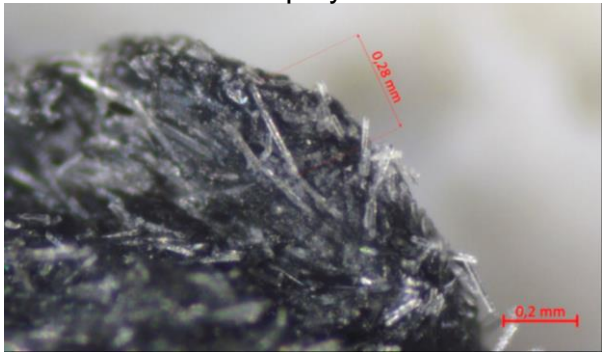
Glass fibers in polymer matrix
